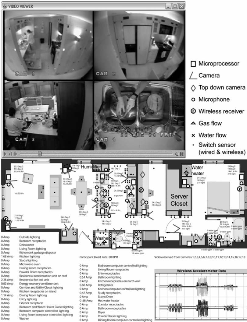
Fig. 3. A data visualization tool for the PlaceLab and a floor plan indicating the location of most sensors described in the text. Data from two wireless 3-axis accelerometers outputting data at 67 Hz is also represented. The display shows the 4 views that were automatically selected from the 18 possible video streams, using computer vision processing. An annotation tool allows researchers to click on a particular sensor and then see the rest of the data (including video and audio) at the time of that sensor’s activation – this may simplify data analysis or searching for particular events of interest in multiple days of data.
