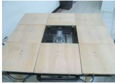
Fig. 3. Embedded RFID and weighing table surfaces
