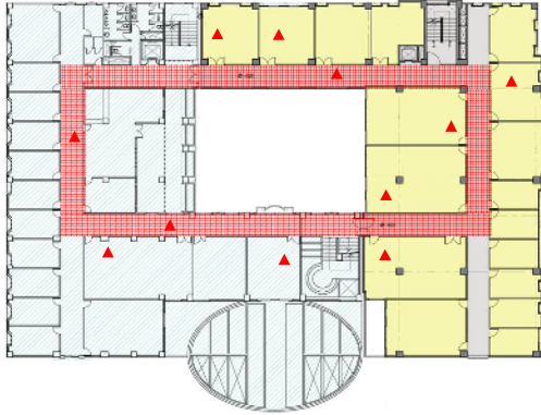
Fig. 6. Floor layout for the experiments. The red triangles are locations of IEEE 802.11 AP and the rectangular area is the corridors of the floor.
